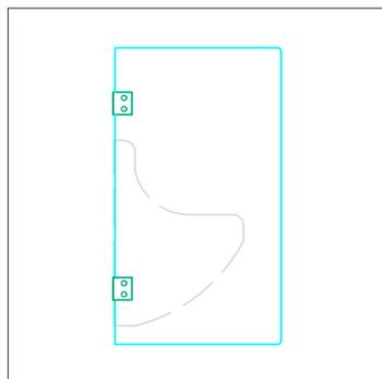
SCHAMWAND MIT KLEMMSCHIENE
