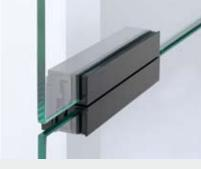
GM BRACKET P is a discreet glass edge securing system for the fixture of glass elements. The system is designed for glass thicknesses of 8 to 12 mm. Due to the possible surface options (standard RAL coatings or eloxal coatings), the system can be colour-coordinated.
